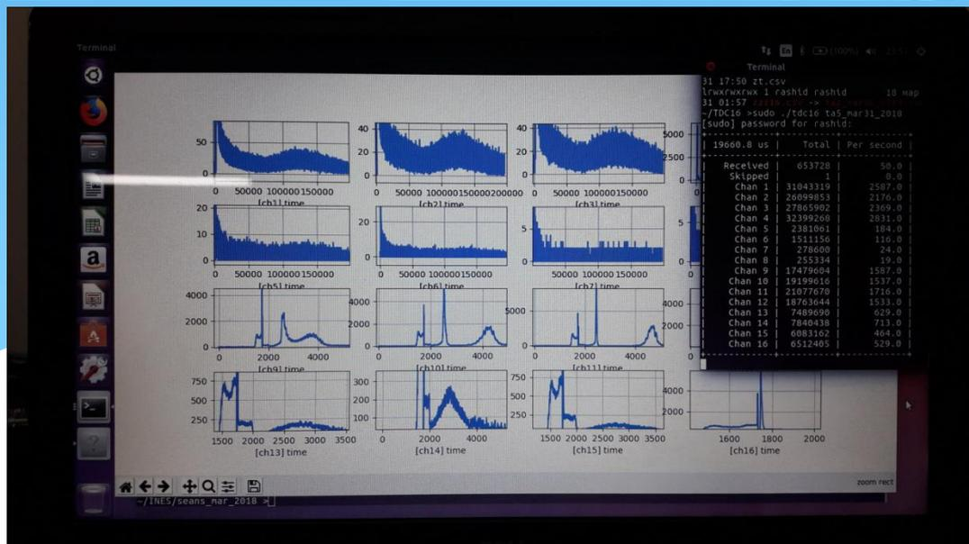
New 16-channel multiplicity data acquisition system was tested at first using  $Co^{60}$  gamma source and  $Cf^{252}$  spontaneous fission neutron source, then it was tested on pulsed beam.
