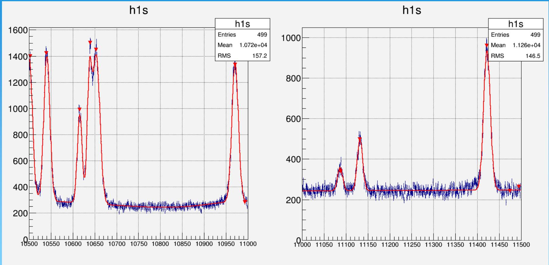
Experimental spectral histograms can be transformed into cross section curves by main two methods. Below few hundreds eV for heavy atoms with high resonance level densities, where  $\Delta E$  of spectrometer resolution function is smaller than  $\Gamma_\gamma$  which is about 0.1 eV, the method of form can be used. At higher neutron energies in the resolved area it's necessary to use method of square areas.
