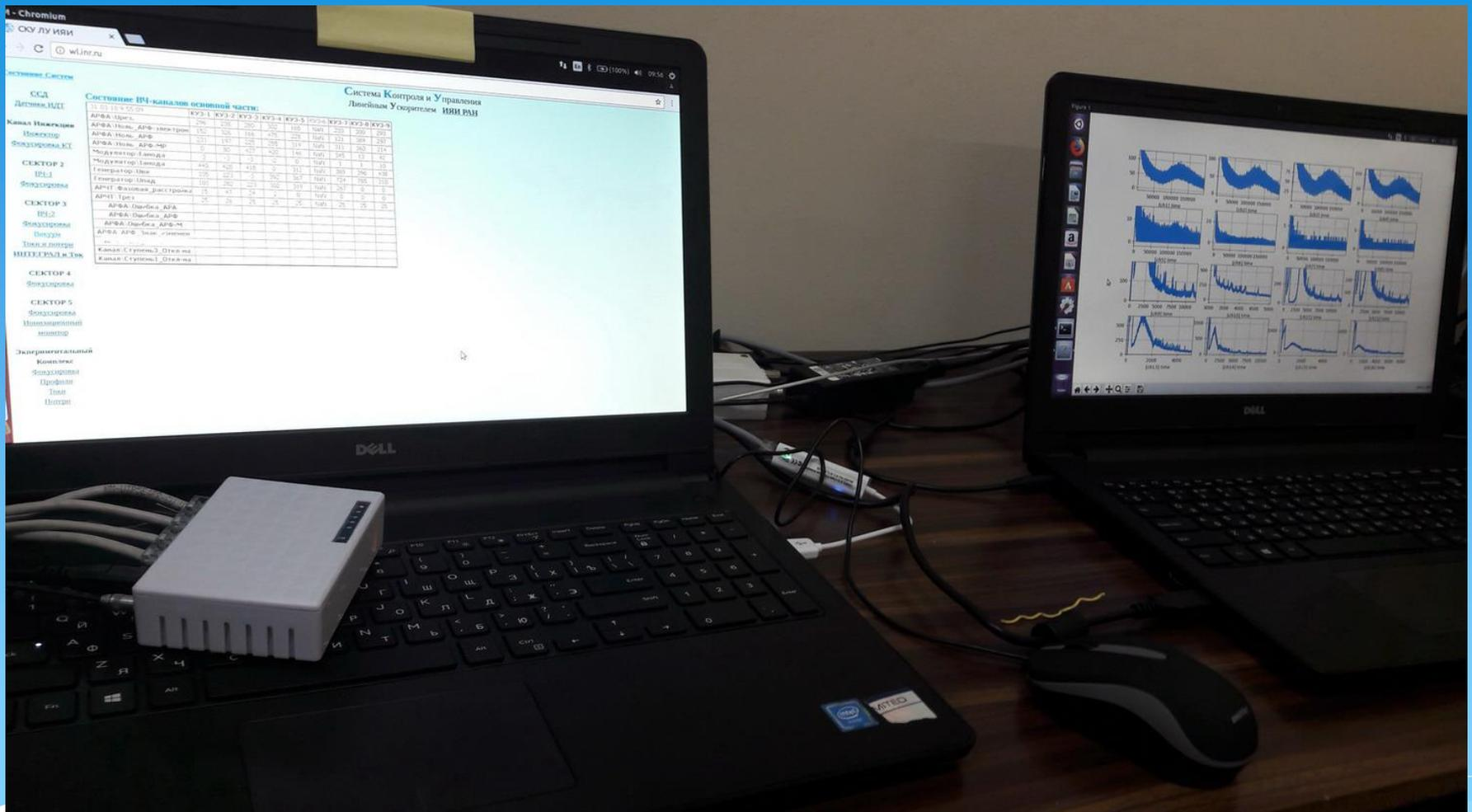
Software for new 16 channel multiplicity data acquisition system is also written in our group using PYTHON. Program allows to interactively observe data on all 16 channels in detail.
